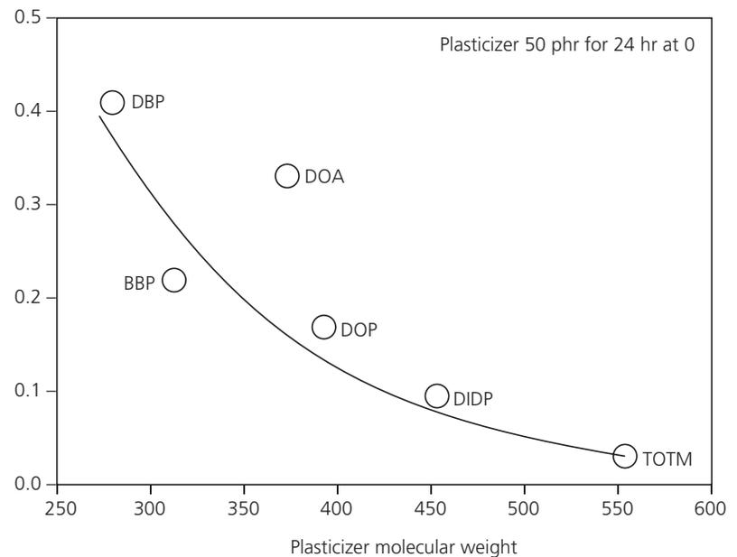
**Figure 4.** Relationship between plasticizer molecular weight and plasticizer migration into polyurethane foam.
