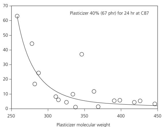
**Figure 2. Relationship between plasticizer molecular weight and volatile plasticizer loss.**
