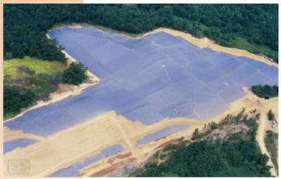
to fit the irregular shape of the waste containment area. Most panels were 20,000 sq. ft. each.
